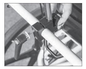
**5.** Unscrew ratchet handle until there is room to insert the head support stem. Insert head support stem.
