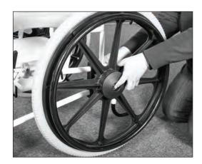
**21.** Using a wrench, loosen the nut on the wheel lock mount and position the wheel lock just in front of the wheel approximately 3/4"-1". Tighten nut securely.
