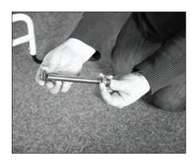
**19.** Depress button on the axle end to recess the ball locking pins, and start the bolt thru the wheel. Place washer on bolt end to inside of wheel.
