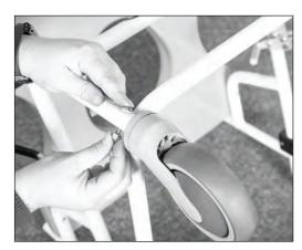
**9.** Use a wrench and hex key to tighten the casters into place.
