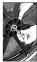
**20.** Continue depressing the button to insert the bolt into the wheel mount.
