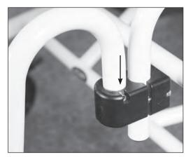
**30.** If the 1-piece foot plate/leg rest was ordered, loosen screw on front anti-tippers clamp.
