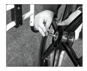
**17**. Insert bolt thru wheel mount. Place spring washer and then nut onto bolt end. Tighten securely.
