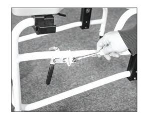
**11.** Turn until the handle is upright as shown, move forward to make room for the wheels and tighten snug. This will be moved once the wheels are on.
